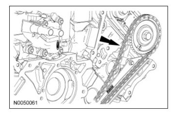
87. Remove the 2 bolts and the LH primary timing chain guide.
