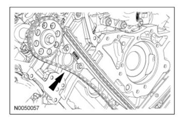
83. Remove the 2 bolts and the RH primary timing chain guide.
