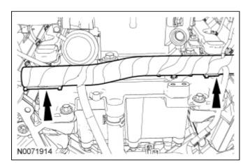
38. Disconnect the PCV valve electrical connector.
