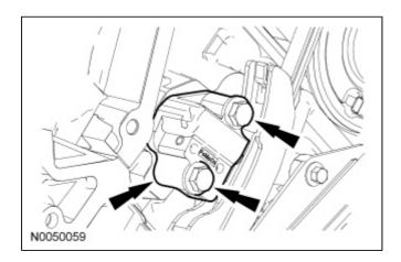
85. Remove the LH primary timing chain tensioner arm.
