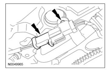
35. Disconnect the bubbler tube from the  $\underline{SC}$ .
