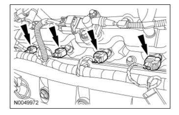
40. Disconnect the fuel rail pressure and temperature sensor electrical connector.
