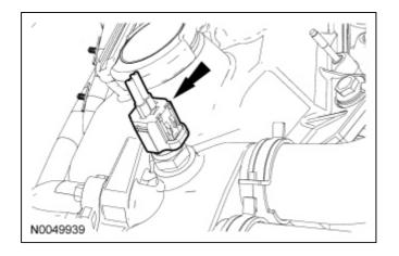
11. Remove the 2 nuts and the thermostat housing assembly.
