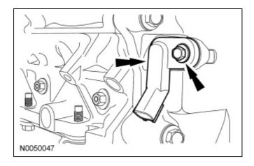
67. Remove the bolt and the <u>CMP</u> sensor.
