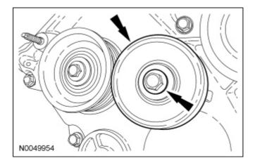
25. Remove the 4 bolts and the coolant pump pulley.
