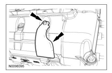
46. Remove the bolt, stud bolt and the RH coil-on-plug cover.
