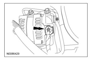
21. Remove the stud bolt, 2 bolts and the alternator.
