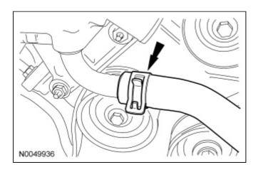
7. Remove the coolant tube bracket nut.
