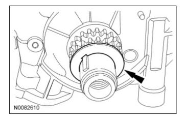
80. Remove the 2 bolts and the RH primary timing chain tensioner.
