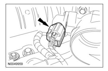
30. Disconnect the Throttle Body (TB) control electrical connector.
