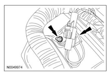
42. Disconnect the EGR valve electrical connector.
