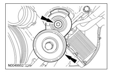
23. Remove the stud bolt and the accessory drive belt idler pulley (smooth).
