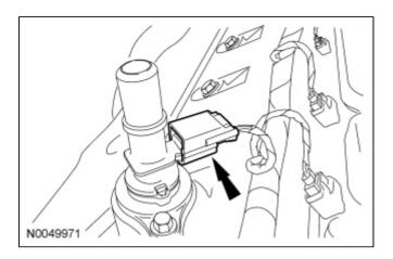
39. Disconnect the 4 RH fuel injector electrical connectors.
