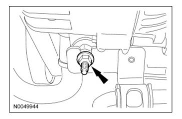
17. Remove the power steering tube bracket bolt.
