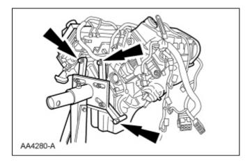
6. Disconnect the coolant hose from the thermostat housing.
