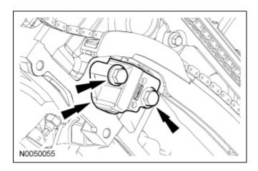
81. Remove the RH primary timing chain tensioner arm.
