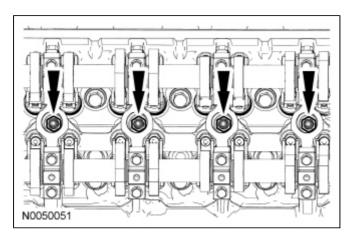
75. NOTICE: If the components are to be reinstalled, they must be installed in their original positions. Mark the components for installation into their original locations. Failure to follow these instructions may result in engine damage.
