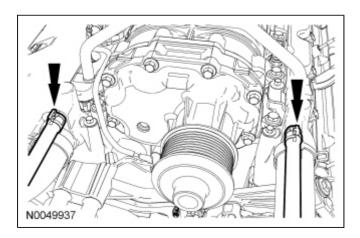
9. Disconnect the 2 upper radiator hoses from the intake manifold.
