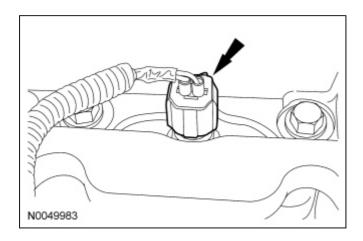
51. Disconnect the 4 LH fuel injector electrical connectors.
