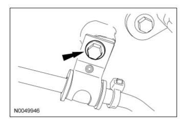
18. Remove the 2 power steering reservoir bracket bolts.
