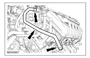
28. Disconnect and remove the crankcase ventilation tube.
