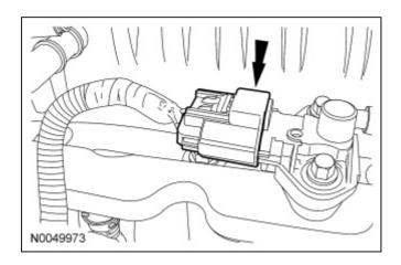
41. Remove the nut and the RH radio interference capacitor.
