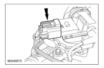
43. Detach the wiring harness from the RH coil-on-plug cover stud bolt.
