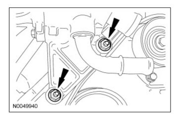
12. Disconnect the coolant hose from the Charge Air Cooler (CAC).
