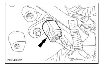
50. Disconnect the Intake Air Temperature 2 (IAT2) sensor electrical connector.
