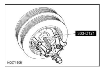
71. Using the Crankshaft Front Oil Seal Remover, remove the crankshaft front seal.
