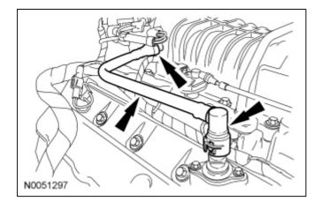
29. Disconnect the <u>TP</u> sensor electrical connector.
