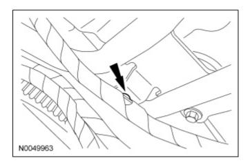
34. Disconnect the LH Heated Oxygen Sensor (HO2S) electrical connector and pin-type retainer.
