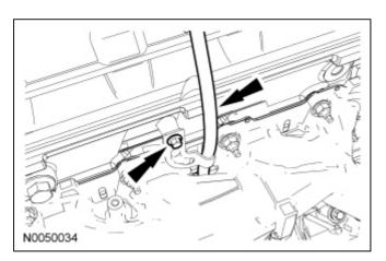
63. **NOTE:** The RH engine support insulator bracket must be removed to access the RH block drain plug.
