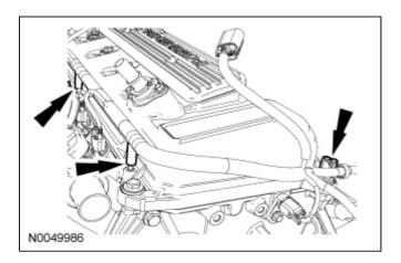
54. Remove the 2 bolts and the LH coil-on-plug cover.
