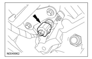
33. Detach the 2 wiring harness pin-type retainers (1 shown) from the coolant tube assembly bracket.
