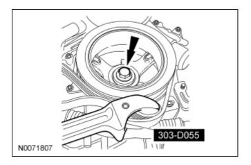
70. Using the 3 Jaw Puller, remove the crankshaft pulley.
