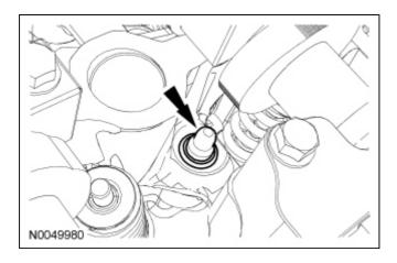
78. Remove the crankshaft sensor ring.
