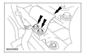
37. Detach the 2 wiring harness pin-type retainers.
