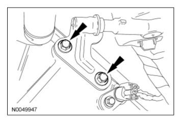
19. Remove the 3 bolts and the power steering pump and reservoir assembly.
