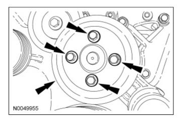
26. Remove the 3 bolts and the 3 <u>SC</u> drive belt idler pulleys.
