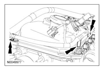
45. Remove the nut and the A/C tube support bracket.
