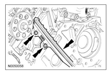
84. Remove the 2 bolts and the LH primary timing chain tensioner.
