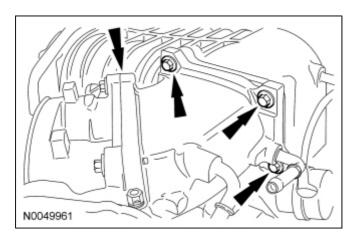
32. Disconnect the Cylinder Head Temperature (CHT) sensor electrical connector.
