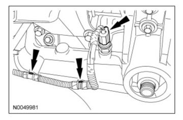
49. Disconnect the Camshaft Position (CMP) sensor electrical connector.
