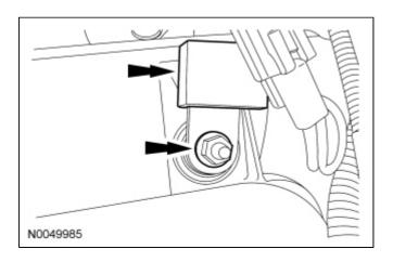
53. Detach the wiring harness retainers from the LH valve cover stud bolts.
