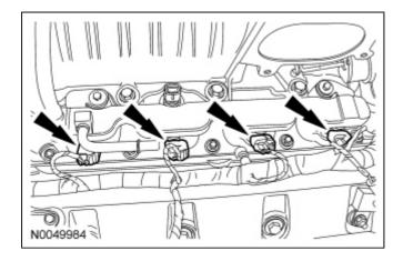
52. Remove the nut and the LH radio interference capacitor.
