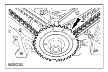
79. Remove the crankshaft washer.
