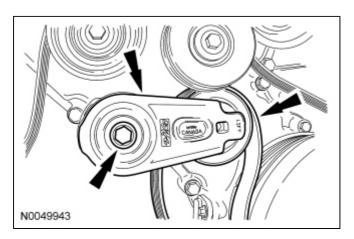
16. Remove the power steering tube bracket nut.
