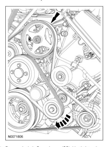
15. Remove the bolt, Supercharger (SC) drive belt tensioner and the <u>SC</u> drive belt.
