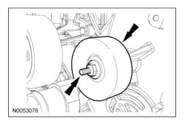
24. Remove the bolt and the accessory drive belt idler pulley (grooved).
