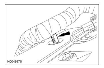
44. Detach the wiring harness retainers from the RH valve cover stud bolts.
